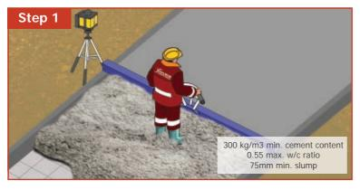
Place, compact & level concrete. Protect from wind, sun and rapid drying.
