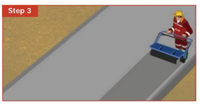
Immediately the concrete can take a mason's weight (slight foot imprint <3mm). Use a dry shake spreader and spread approx 50% of X-Tech IntegraFloor.
