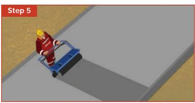
As soon as Step 4 has started follow with the second application of X-Tech IntegraFloor. Apply at a right angle to the first application.
